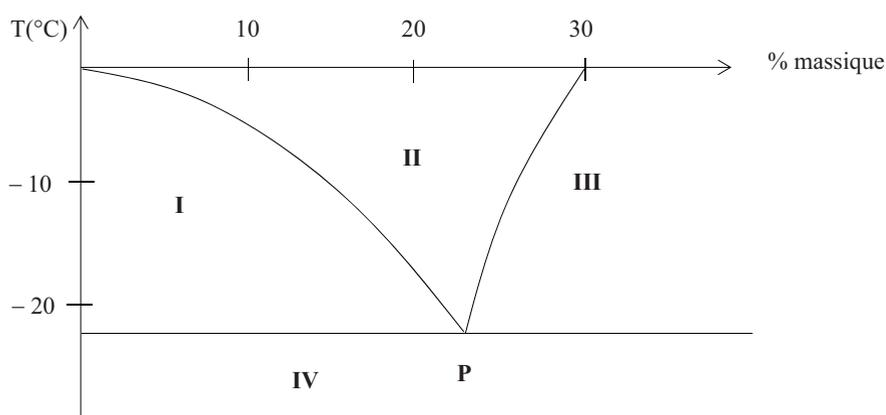
Figure 9 - Diagramme binaire (eau-NaCl)
