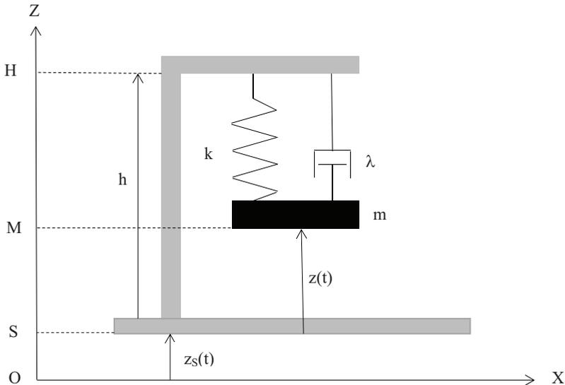
Figure 1 - Sismographe
