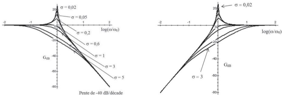
$$\underline{H}(j\omega) = \frac{H_0}{1 + 2j\sigma \frac{\omega}{\omega_0} + \left(\frac{j\omega}{\omega_0}\right)^2}$$
