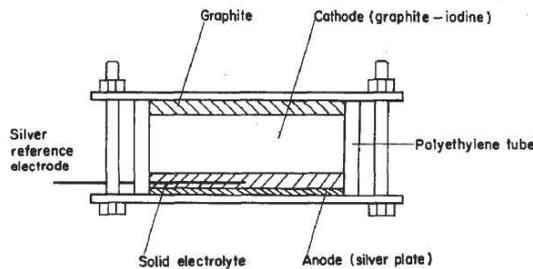
Figure 7: prototype de la pile  $Ag/Ag_3SI/I_2$ .
