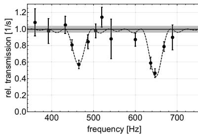
**Figure 9** Taux de transmission des neutrons en fonction de la fréquence. Figure extraite de G. Cronenberg et al., *A Gravity of Earth measurement with a qBounce experiment*, Proceedings of the EPS Conference on High Energy Physics 2015, arXiv : 1512.09134
