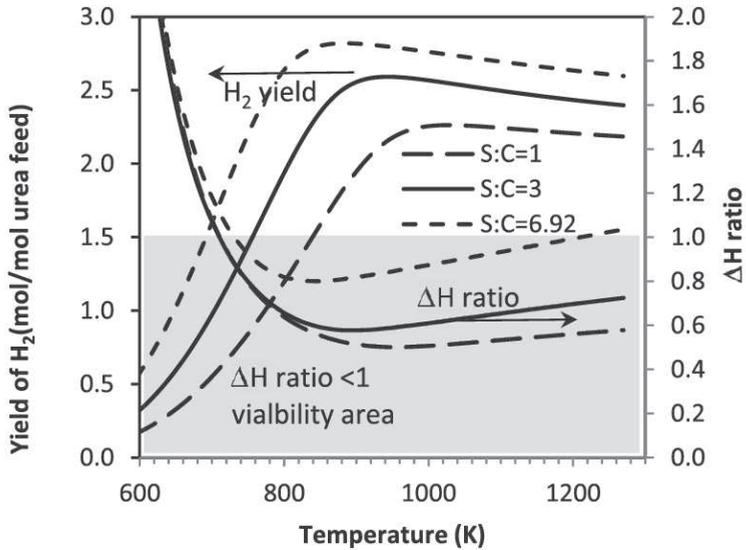
Fig. 2 – Effect of S:C ratio on H<sub>2</sub> yield and  $\Delta H$  ratio with reaction temperature.
