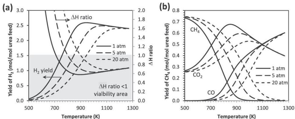
Fig. 6 – Effect of pressure on (a)  $H_2$  yield and  $\Delta H$  ratio (b) Carbon products yield for  $S:C = 3$ . Calculations performed without  $CaO_{(s)}$  in the reactants, and without  $C_{(s)}$  in the products.
